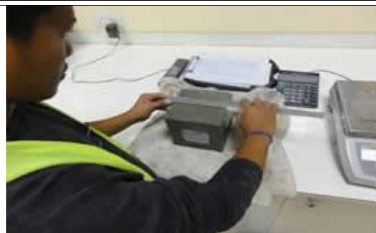
Checking the dimensions of the Concrete Cube Specimens prior of weighing & crushing
