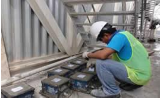
Markings or Identification for the newly casted (molded) Concrete Cube Specimens
