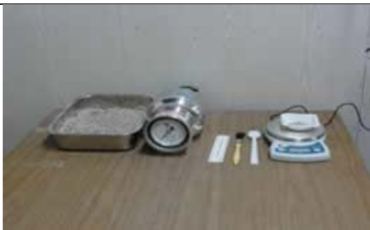
Moisture Content Determination with the use of Speedy Moisture Tester
