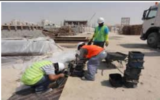
Casting of Concrete Cubes Specimens 150mm x 150mm x 150mm (Molding of Strength Specimens)
