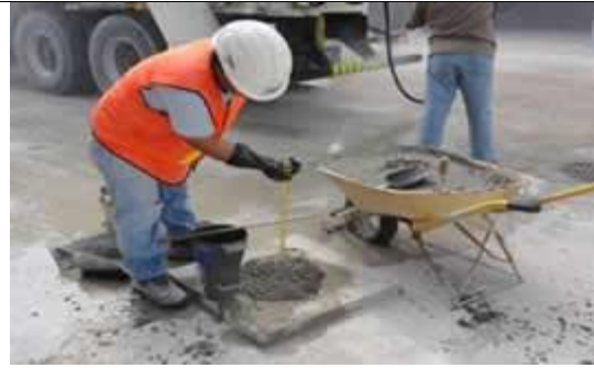
Performing the Slump Test for the Freshly Mixed Concrete
