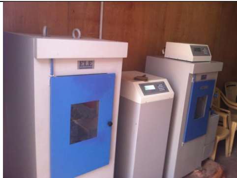
CUBE TESTING MACHINES ON SITE 3000 KN CAPACITY
