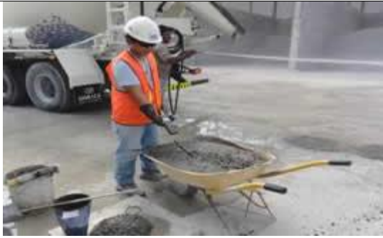
Checking the Temperature of Freshly Mixed Concrete
