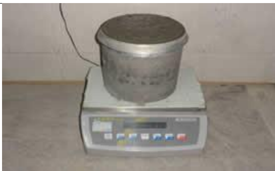
Checking the Plastic Density (Unit Weight & Yield) of the Freshly Mixed Concrete
