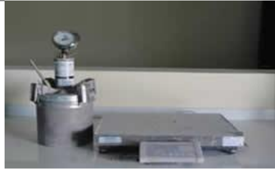
Air Entrainment Meter Weighing Scale or Balance (Test Conducted at Basra University)
