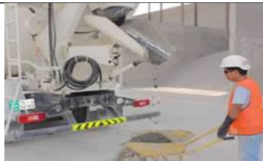
Sampling of Freshly Mixed Concrete from the Transit Mixer For Al Yamama Batching Plant Mix QA/QC assurance
