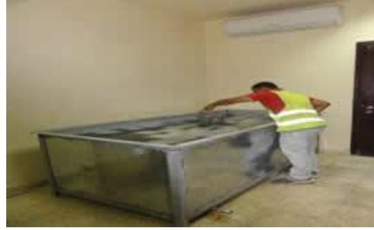
Curing Tank for the casted Concrete Specimens in the laboratory
