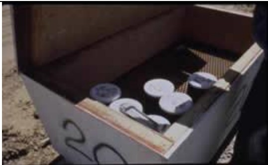
Curing Tank for the casted Concrete Specimens in the field
