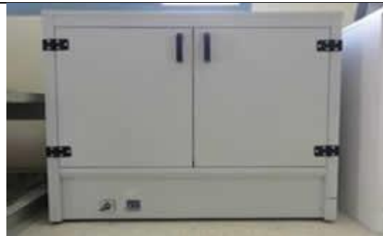
Moisture Content Determination with the use of Thermostatic Drying Oven
