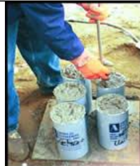
Casting of Concrete Cylinders Specimens 150mm x 300mm (Molding of Strength Specimens)
