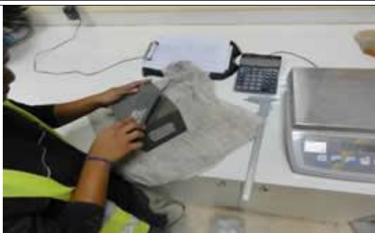
Removal any surface fins from the Concrete Cube Specimen using the grinding stone
