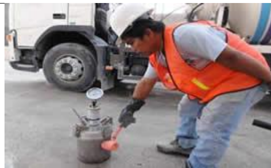
Checking the Air Content for the Freshly Mixed Concrete using Air Entrainment Meter
